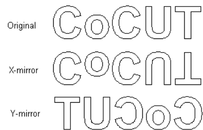
Fig. 47: Example of the Mirror Command
