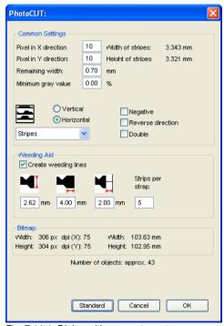
Fig. 7.11-1: Dialog with parameter-setup
