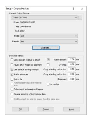
Clicking the Calibrate button opens the Calibrate Device dialog.
