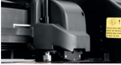
Fig. 4.10-4: Cutting head with sensor and tangential knife
